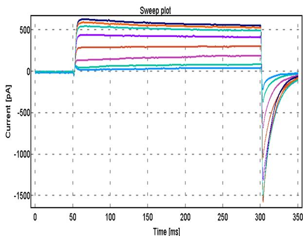
**Fig. 3.1.6.3:** Long time course of a CHO K<sub>v</sub>1.6 cell. Peak current amplitude was reduced by increasing concentrations of 4-AP.
